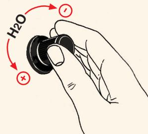
Start at the lowest end and gradually build water intensity. Inadequate water will produce a spluttering, intermittent stream. Use only enough water for a steady stream.
